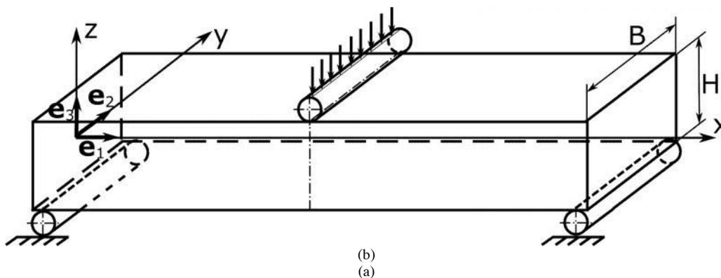
Figure 1: Geometry of the three-bending test. Diameter of loading (supporting) cylinders is  $d$ .
