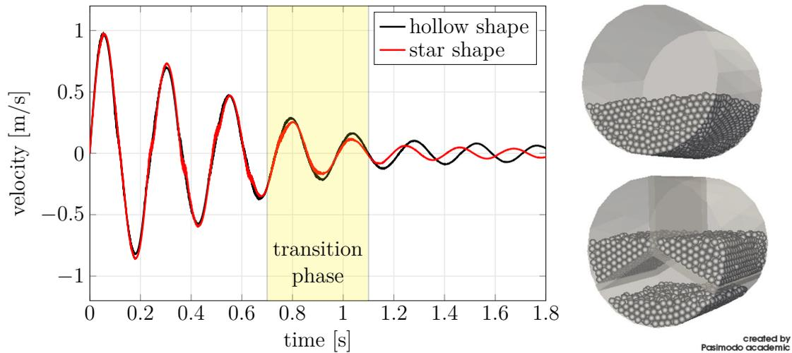
Figure 1: Simulation results comparing the damping performance of two different container geometries (left). Star shaped internal geometry (bottom-right) and hollow geometry (top-right).
