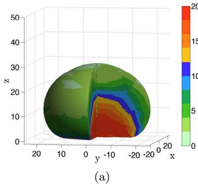
Figure 1: Example of the impact of a sphere on a rigid ground, approximated with a Nitsche-based method.
