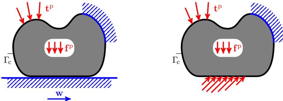
Figure 2: The steady sliding frictional contact problem for a continuum.
