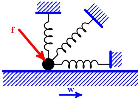
Figure 1: The steady sliding frictional contact problem for a point particle.
