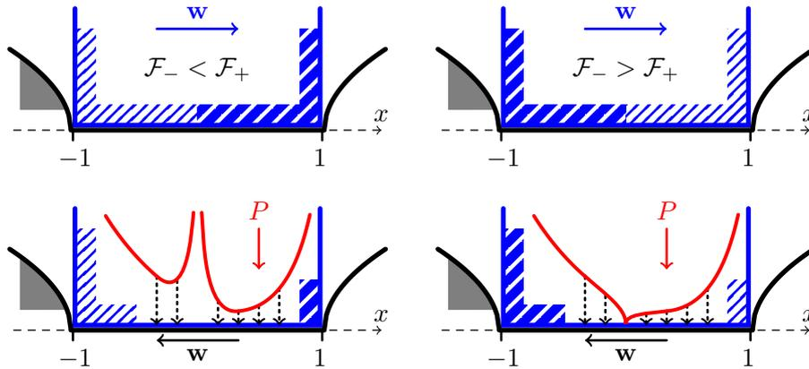
Figure 3: Normal component of the surface traction when the larger friction coefficient is front (left) or rear (right).
