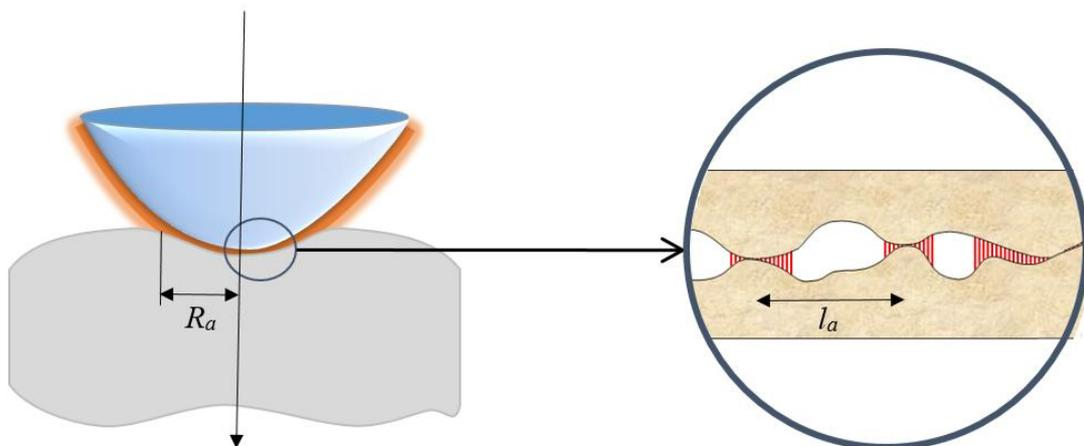
Figure 1: Scheme of contact at two scale levels.
