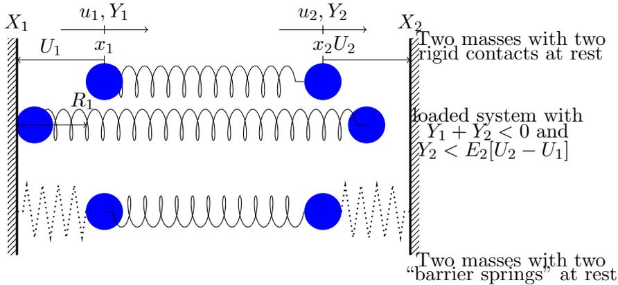
Figure 2: Two masses with 2 rigid contacts, loads  $Y_1, Y_2$
