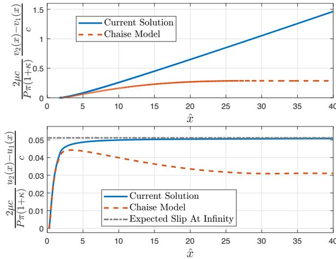
Figure 2: For  $f = 0.5$ , **Top:** Separation along the contact interface. **Bottom:** Relative slip along the interface. Results from the current model are compared with the results from the Chaise model.
