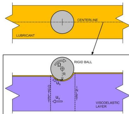
Figure 1: schematic of the problem studied in the lubricated case. A rigid sphere rolls over a linearly viscoelastic layer.
