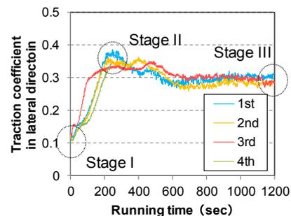
Figure 3: Change of traction coefficient in lateral direction with running time
