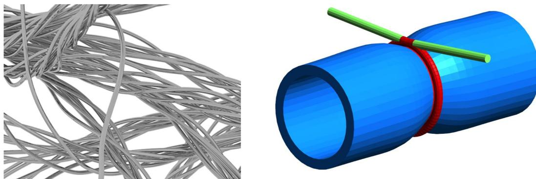
Figure 1: Beam-to-beam contact (left) and beam-to-solid contact (right).
