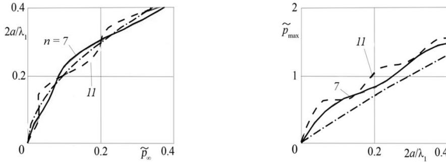
Figure 1: Dimensionless contact pressure versus contact length at different  $n$  in comparison with single cosine profile (dash-dot line): (a) nominal pressure, (b) maximum pressure.
