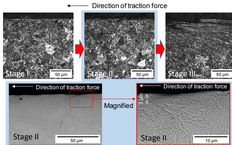
Figure 5: Metallic structures measured by optical and scanning electron microscope.
