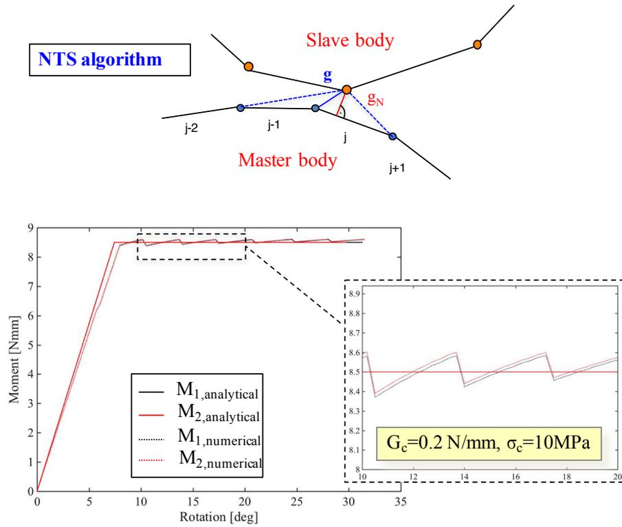
Figure 1: Global response of a Moment Loaded DCB in mode-I loading condition.
