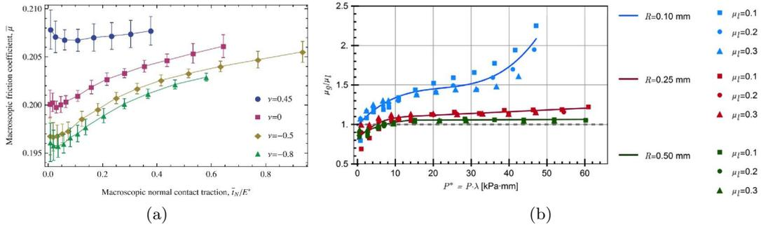
Figure 2: Macroscopic friction-pressure relationship: (a) in Case 1, for different values of Poisson ratio  $\nu$ , (b) in Case 2, for different cylinder radii  $R$  and different local friction coefficient  $\mu_l$ .
