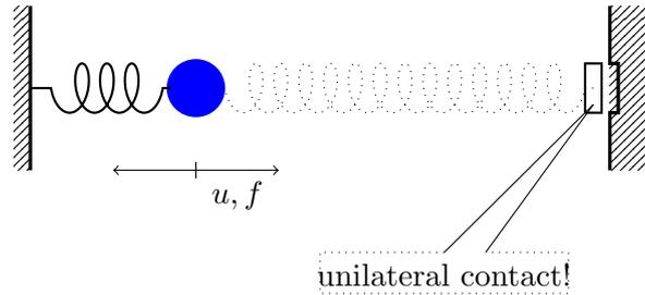
Figure 1: One mass with 2 springs with a weak unilateral one, load  $f$
