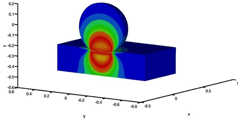
Figure 1 : 3D numerical Hertz contact with contour plot of Von Mises stress.
