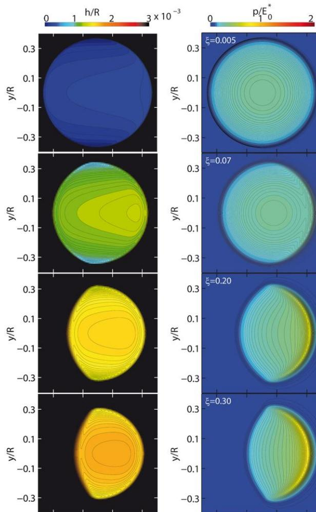
Figure 2: Contour plots of the film thickness (left) and the pressure distribution (right) for different values of the dimensionless speed.
