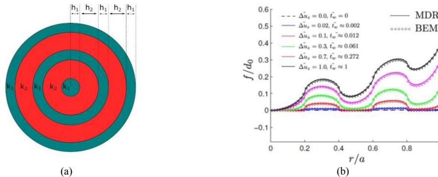
Figure 1: Wear of an annular cylinder (a) with 5 rings having different wear coefficient  $k_2/k_1=10$ , (b) worn profiles during the wear process (ratio of ring width  $h_2/h_1=1$ ).
