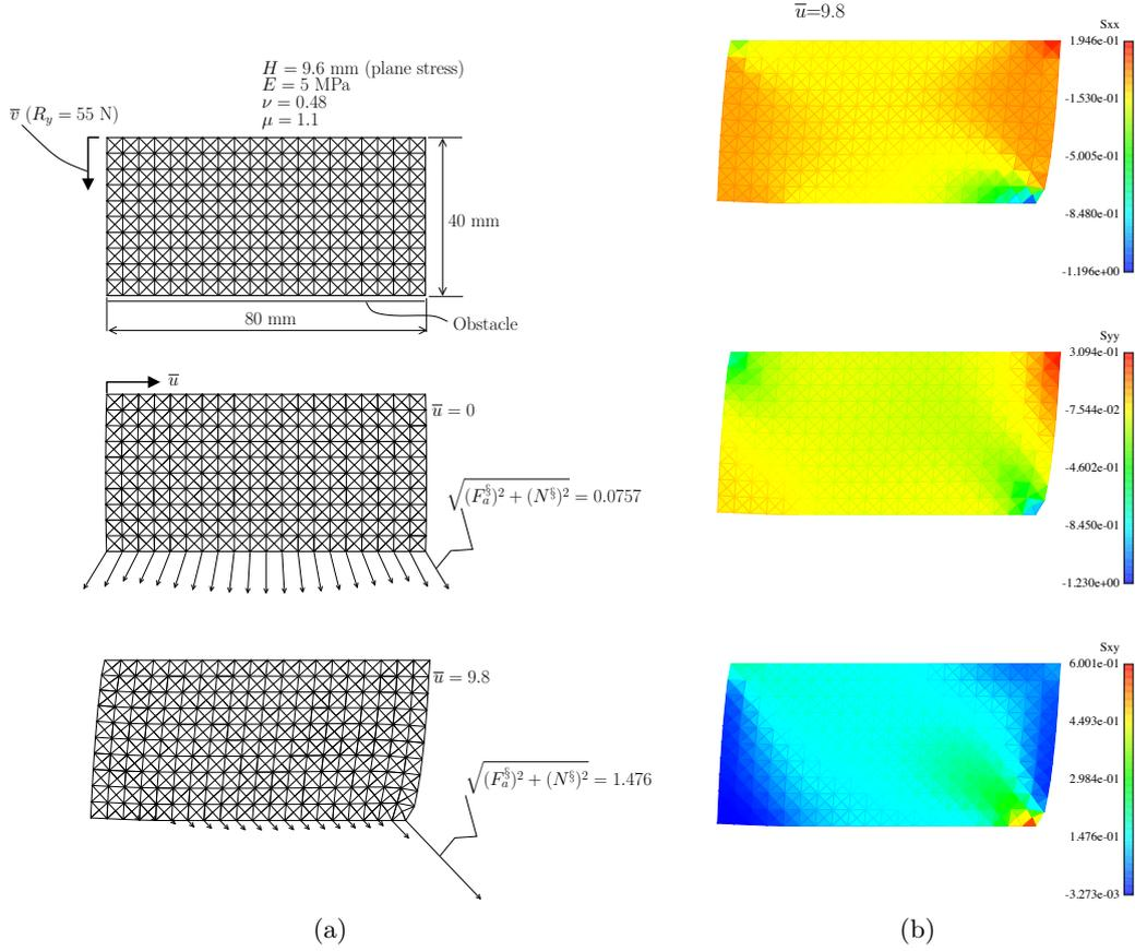
Figure 1: A tangentially driven elastic discretized block: (a) Finite element mesh, type of loading and actions on the obstacle, (b)  $\sigma_{xx}$ ,  $\sigma_{yy}$  and  $\sigma_{xy}$  (MPa) components of the Cauchy stress tensor during the steady sliding regime.
