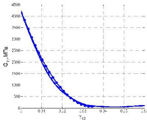
Figure 2: Experimental results: softening of the core for shear stresses.
