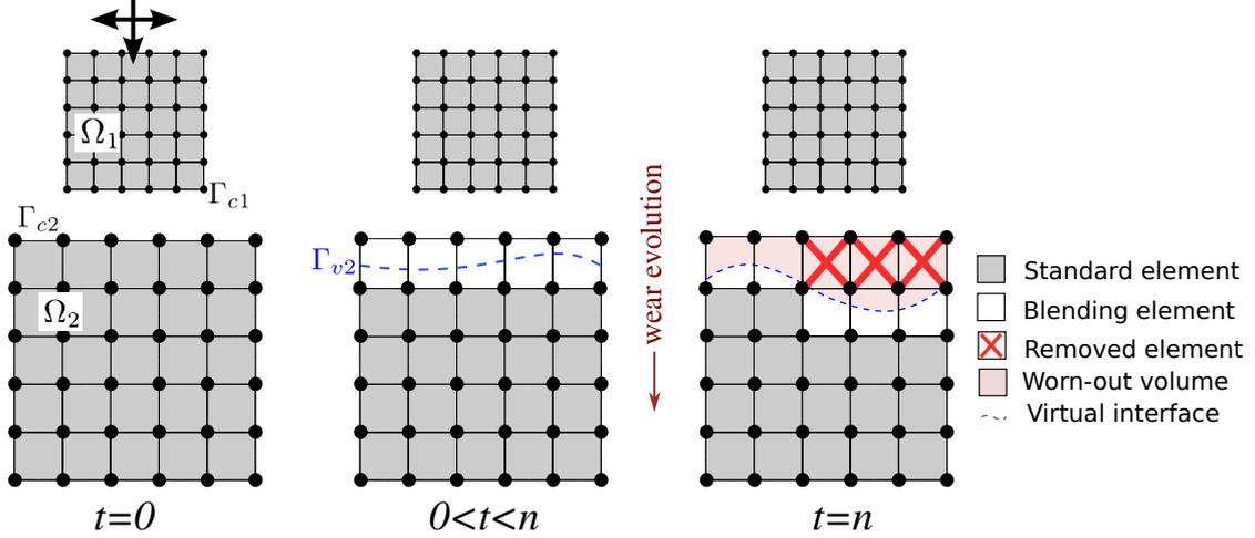
Figure 1: Wear at the interface, modeled using virtual interface  $\Gamma_v$  (total simulation time  $t = n$ ).
