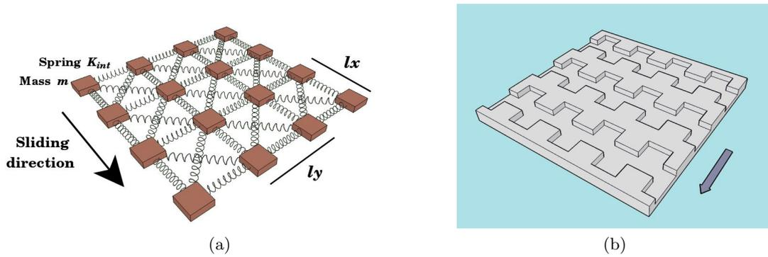
Figure 1: (a) Discretization of a square surface into a 2-D spring-block model, showing the mesh of the internal springs. (b) Example of winding tread patterns analyzed with the spring-block model allowing to reduce the static friction coefficient.
