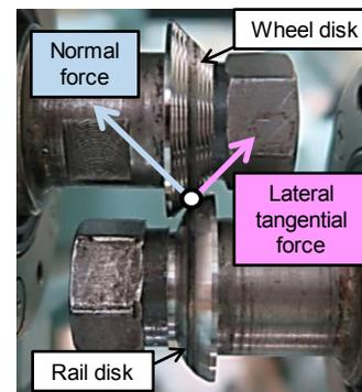
Figure 2: A set of wheel disk and rail disks after attachment on the experimental apparatus
