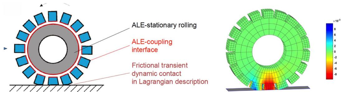
Figure 1: left) principle sketch of the Lagrangian - ALE coupling scheme for rolling contact of treaded tires; right) on a simplified test structure computed displacement field.
