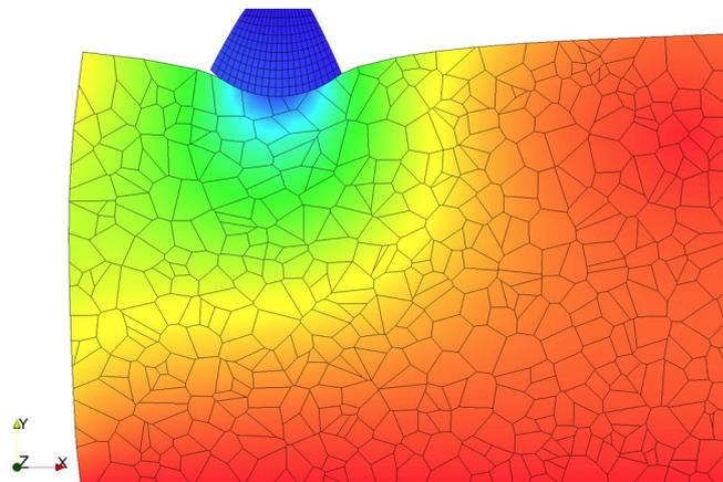
Figure 1: Ironing problem using an arbitrary mesh with complex element shapes.
