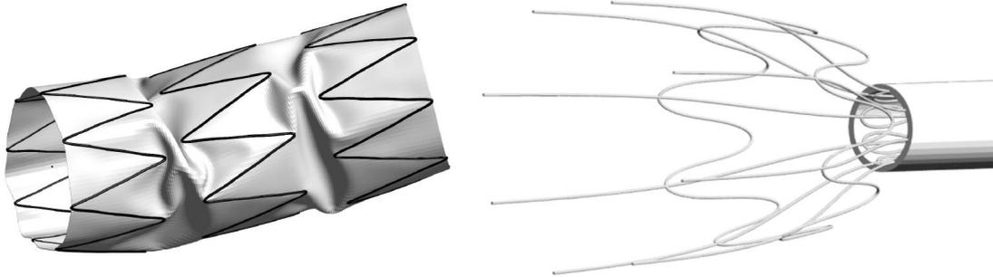
Figure 2: Beam-to-solid interaction: stent graft as an example for mesh tying (left) and bare-metal stent in catheter as an example for contact (right).
