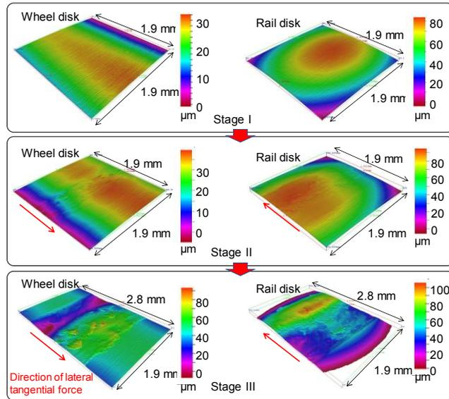
Figure 4: Change of surface topography of wheel disk and rail disk for different stage.
