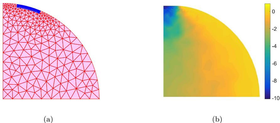
Figure 1: Spherical indentation: (a) finite element global and local meshes in the undeformed configuration, (b)  $\sigma_{yy}$  component of the Cauchy stress tensor in the deformed configuration.
