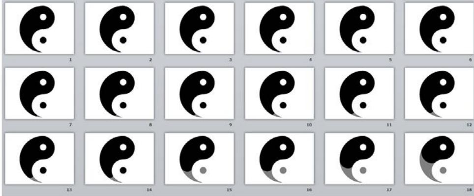
Figure 1: Consecutive phases of detachment of a flat-ended stamp in form of “Yin and Yang”. The last shown configuration is the last stable configuration. After that, the stamp instantaneously detaches completely.
