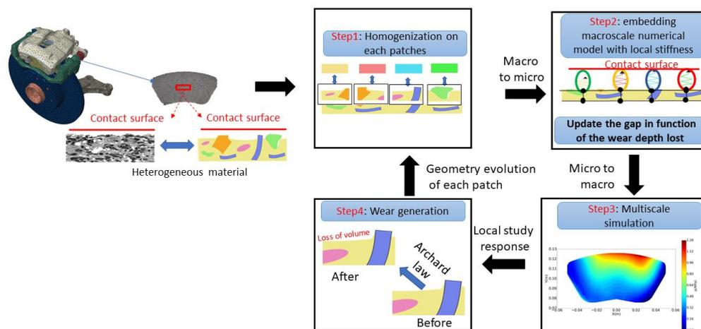
Figure 1: The global strategy showing the wear modeling considering heterogeneous friction material
