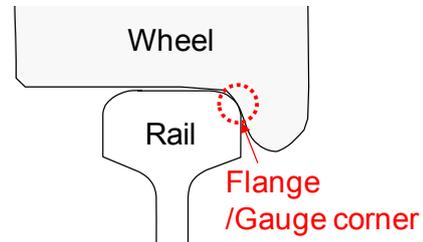
Figure 1: Wheel flange/rail gauge contact position
