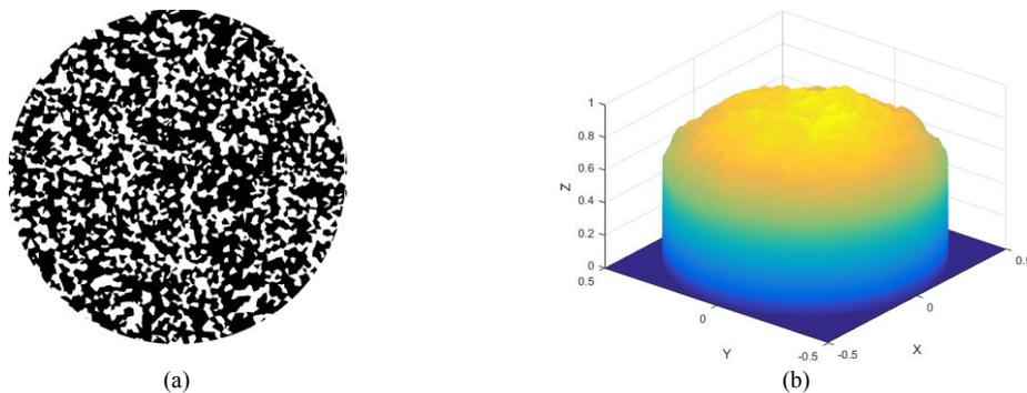
Figure 2: An example of biphasic composite: (a) distribution of two phases with wear coefficient  $k_2/k_1=10$  (white and black); (b) the worn surface topography at the stationary state.
