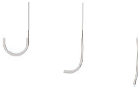
Figure 1: The beam-inside-beam contact framework keeps a string of consecutive beam elements embedded within another string of consecutive beam elements. Left: initial configuration, center: intermediate configuration, right: final configuration.
