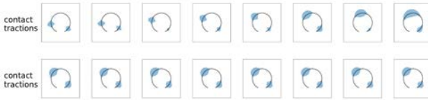
Figure 2: Contact tractions on \Gamma_c^+ at the microscopic level. Dry pores (above) and fluid-filled (bottom) cells Y at macroscopic locations along line D-E, see Fig. 1
