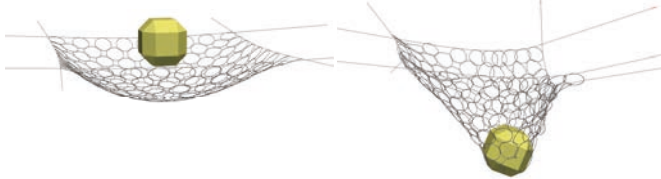
Figure 1: Simulation of rockfall protection ring nets with frictional contact.
